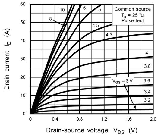
**Fig. 8.2  $I_D - V_{DS}$**
