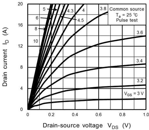
**Fig. 8.1  $I_D - V_{DS}$**
