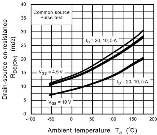
**Fig. 8.9  $R_{DS(ON)} - T_a$**
