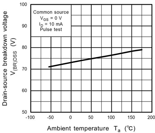
**Fig. 8.11  $V_{(BR)DSS} - T_a$**
