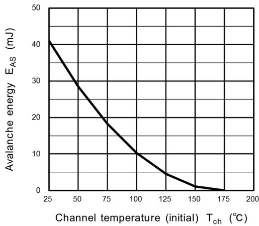
**Fig. 8.15  $E_{AS} - T_{ch}$**
