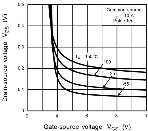
**Fig. 8.3  $V_{DS} - V_{GS}$**
