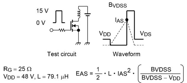
**Fig. 8.16 Test Circuit/Waveform**
