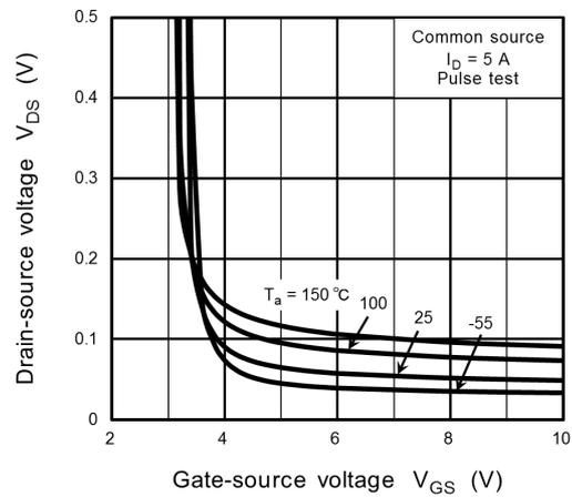
**Fig. 8.4  $V_{DS} - V_{GS}$**
