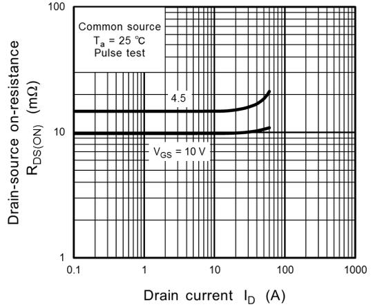
**Fig. 8.8  $R_{DS(ON)} - I_D$**
