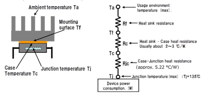
Figure 11 Selecting a heat sink
