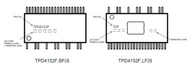
Figure 2 HSSOP31 package typical markings
