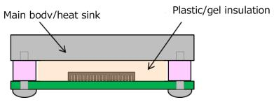
Figure 9 Adding a heat sink using plastic or gel insulation
