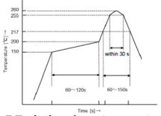
Figure 7 Typical package temperature profile
