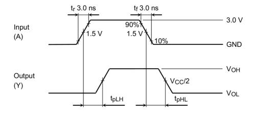
Fig. 11.9.1 t<sub>PLH</sub>, t<sub>PHL</sub>
