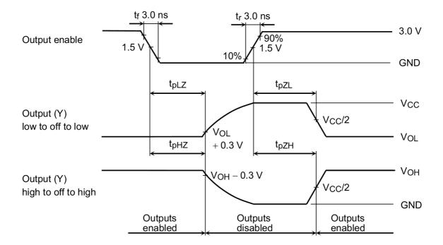
Fig. 11.9.2 t<sub>PLZ</sub>, t<sub>PHZ</sub>, t<sub>PZL</sub>, t<sub>PZH</sub>
