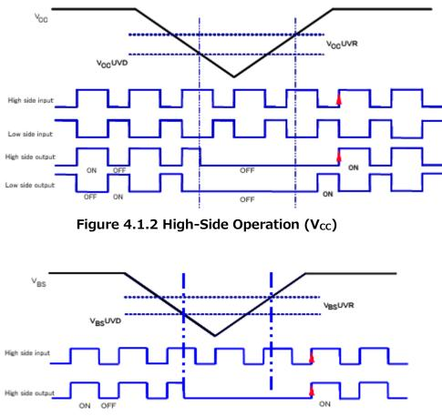
Figure 4.1.3 High-Side Operation (V<sub>BS</sub>)
