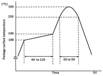
Figure 2.4 Example of a reflow soldering profile
