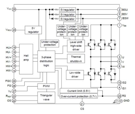
Figure 1.2.1 Block Diagram
