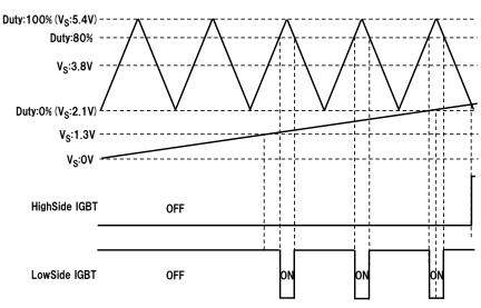
Figure 4.3.1 V<sub>s</sub> and PWM Operation (V<sub>s</sub>=0 V to 2.1 V)
