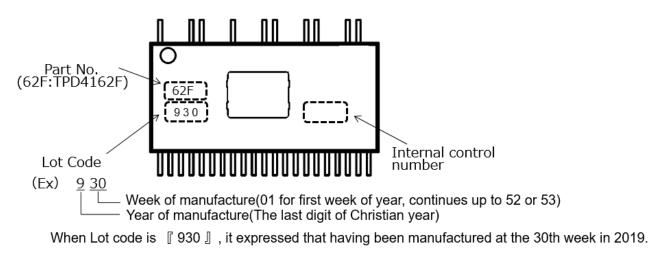
Figure 2.2 Part marking on the HSSOP31 package
