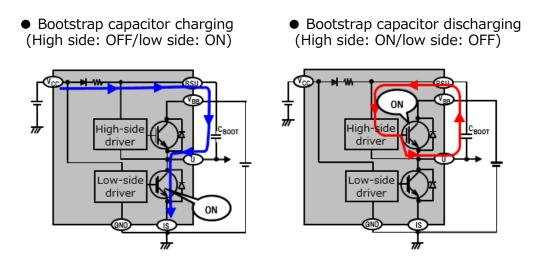
Figure 4.3.2 Bootstrap Capacitor Charge/Discharge Operation ( $V_s$ =1.3 V to 2.1 V)
