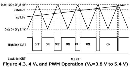
Even if  $3.8V \le V_{S} \le 5.4$  V, the ON-period of the high-side IGBT is determined by comparing the triangle wave and V<sub>S</sub>-voltage as shown above. The low-side IGBT is ALL OFF at 3.8 V $\le$ V<sub>S</sub> (Duty:55 % or more), but PWM control is performed at the high-side IGBT, the diode recovery current flows to the low-side FRD controlled by PWM, and the bootstrap capacitor is charged in the path shown in the figure below.
