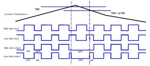
Figure 4.1.4 Thermal shutdown during low-side operation
