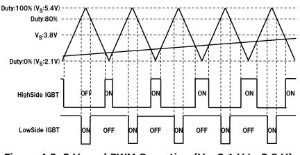
Figure 4.3. 3 V<sub>s</sub> and PWM Operation (V<sub>s</sub>=2.1 V to 3.8 V)
