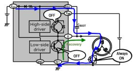
Figure 4.3.5 Bootstrap Capacitor Charge/Discharge Operation ( $V_s$ =3.8 V to 5.4 V)
