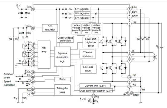
Figure 1.2.2 Example of Application Circuit
