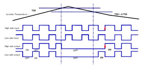
Figure 4.1.5 Thermal shutdown during high-side operation
