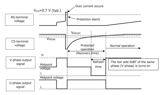
Figure 4.1.7 Timing Chart for Overcurrent Protection Operation
