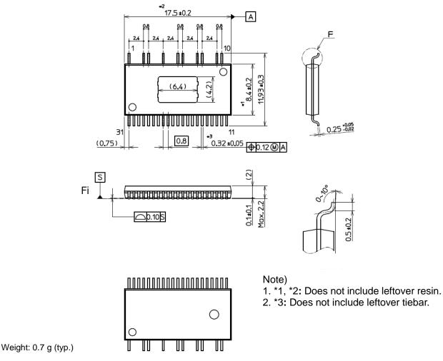
Figure. 2.1 Dimensions of HSSOP31 packages
