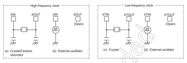
Figure 2-3 Examples of Resonator Connection
