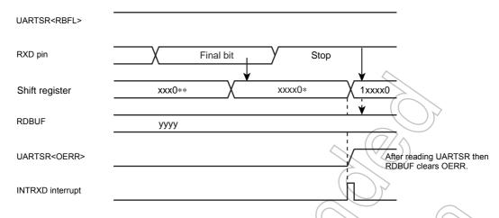
Figure 11-7 Generation of Overrun Error
