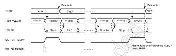
Figure 11-9 Generation of Transmit Data Buffer Empty
