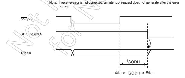
Figure 10-17 Hold Time of the End of Transmit/Receive Mode
