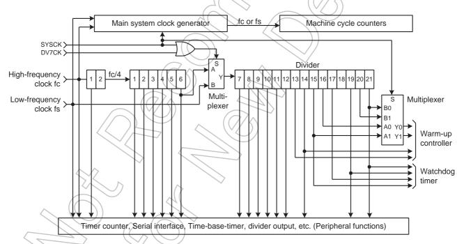
Figure 2-4 Configuration of Timing Generator
