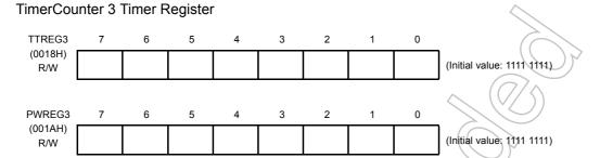
Note 1: Do not change the timer register (TTREG3) setting while the timer is running.
