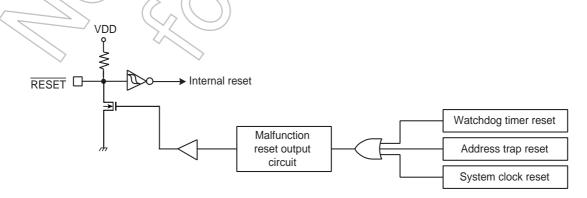
Figure 2-15 Reset Circuit
