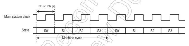
Figure 2-5 Machine Cycle
