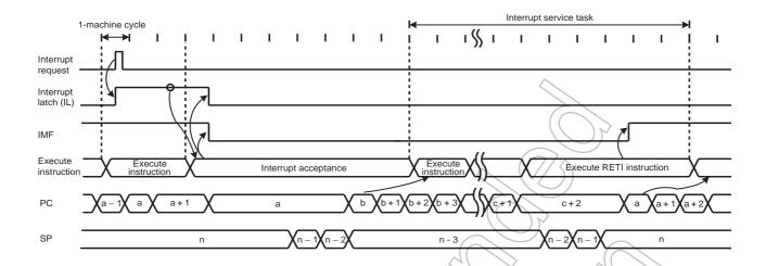
Note 1: a: Return address entry address, b: Entry address, c: Address which RETI instruction is stored.
