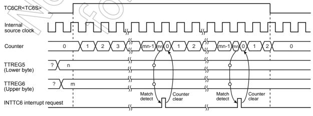
Figure 9-6 16-Bit Timer Mode Timing Chart (TC5 and TC6)
