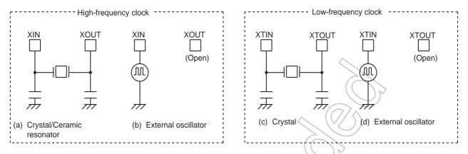
Figure 2-3 Examples of Resonator Connection
