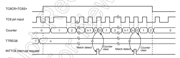
Figure 9-3 8-Bit Event Counter Mode Timing Chart (TC6)
