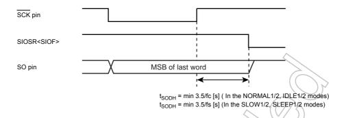
Figure 12-9 Transmiiied Data Hold Time at End of Transfer
