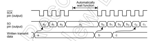
Figure 12-3 Automatic Wait Function (at 4-bit transmit mode)
