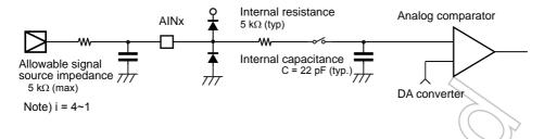
Figure 13-4 Analog Input Equivalent Circuit and Example of Input Pin Processing
