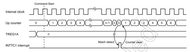
Figure 8-2 Timing chart for timer mode
