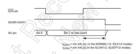
Figure 12-12 Transmitted Data Hold Time at End of Transfer / Receive
