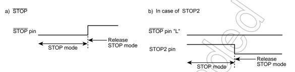
Figure 14-2 Priority of STOP pin and STOP2 pin
