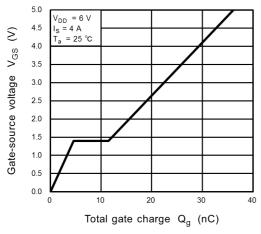
Fig. 9.7 Dynamic Input Characteristics
