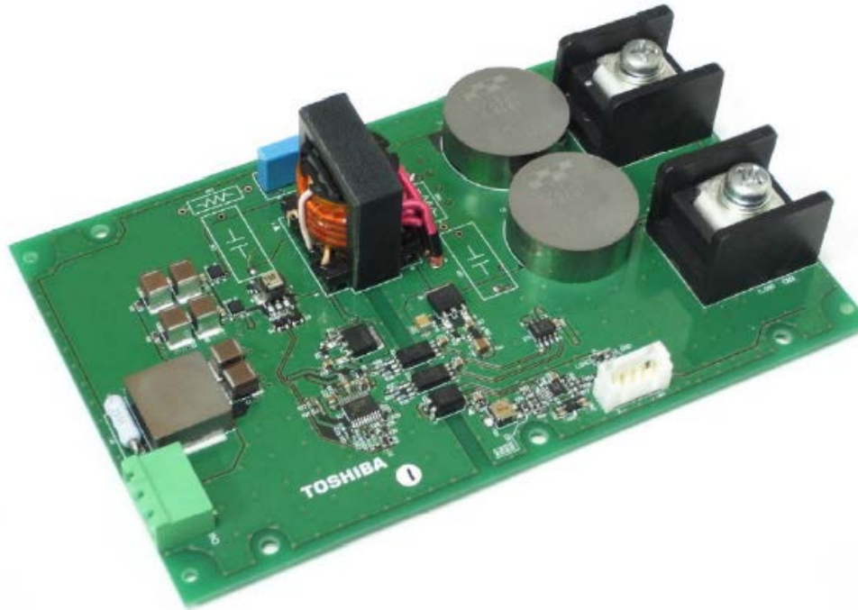
Fig. 1.1 Picture of Half-bridge DC-DC converter evaluation board supporting 48V Bus systems
