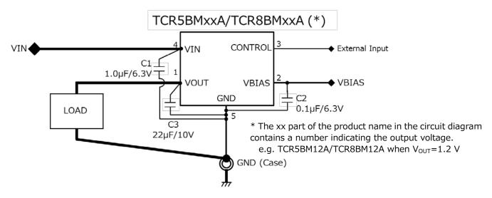
Figure 4.1 Routing Image of Wiring Pattern
