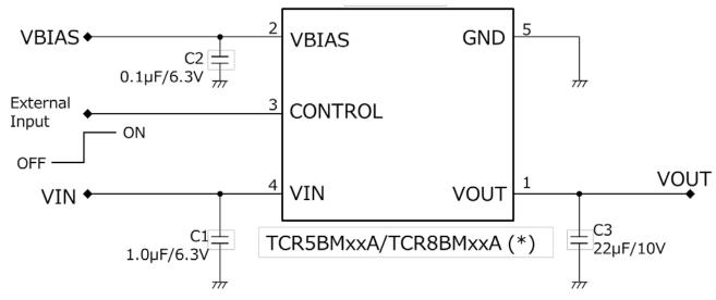
Figure 3.1 Applied Circuits for TCR5BM/TCR8BM Series MCUs
