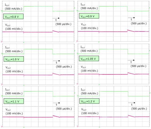
Figure 4.4 Load Transient Responses of TCR5BM Series ( $V_{IN}$ =1.35 V,  $V_{BIAS}$ =3.3 V,  $I_{OUT}$ =1 mA-500 mA-1 mA,  $C_{OUT}$ =22 µF)
