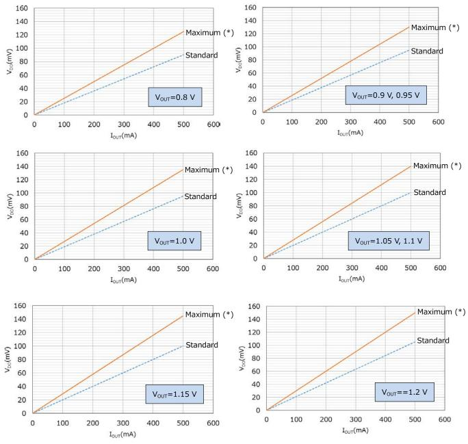
Figure 4.2 Dropout Voltage Characteristics of TCR5BM Series (V<sub>BIAS</sub>=3.3 V, V<sub>OUT</sub>=0.8 to 1.2 V) \* The maximum condition includes the full
