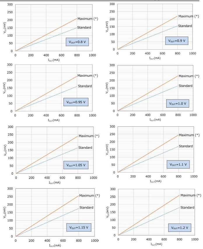
Figure 4.3 TCR8BM Series Dropout Voltage Characteristics (V<sub>BIAS</sub>=3.3 V, V<sub>OUT</sub>=0.8 to 1.2 V)
