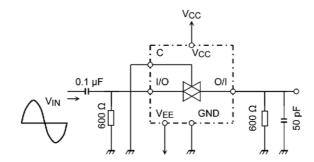
Figure 4 Feedthrough Attenuation
