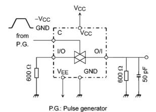
Figure 5 Cross Talk (control input to output signal)
