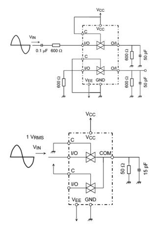
Figure 6 Cross Talk (between any two switches)
