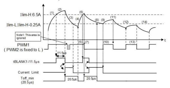
Figure 7.14 Chopper-type current-limit control
