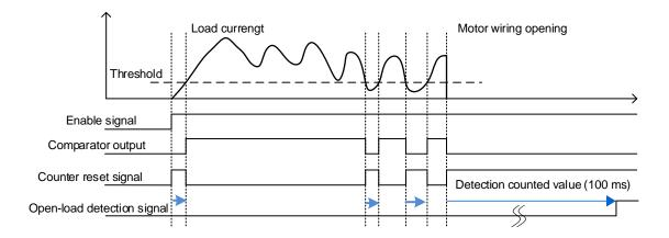
Figure 7.23 Open-load detection during operation: operation waveform
