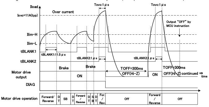
Figure 7.42 Over-current detection operation timing chart 1
