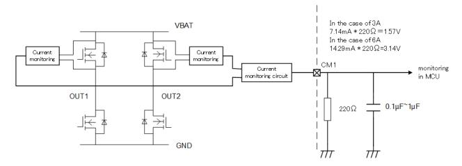
Figure 7.18 High-side current monitoring configuration
