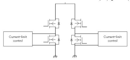
Figure 7.15 Current measurement points in current-limit control
