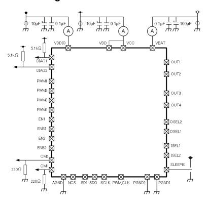
Figure 11.1. Current consumption measurement circuit diagram
