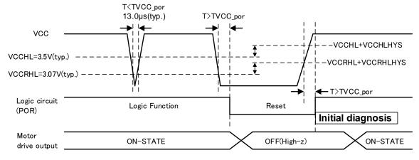
Figure 7.39 VCC under-voltage POR detection timing chart 1
