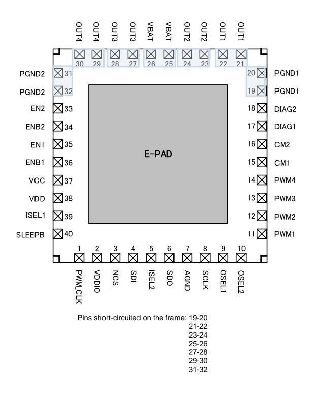
Figure 5.1. Pin assignment
