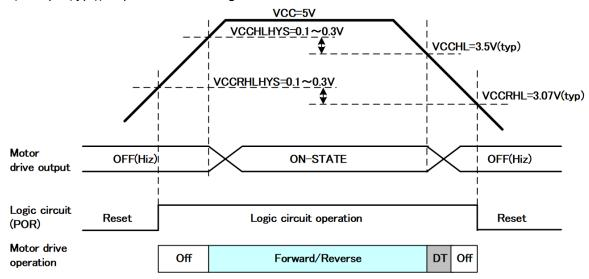
Figure 7.37 VCC under-voltage detection and POR threshold characteristics
