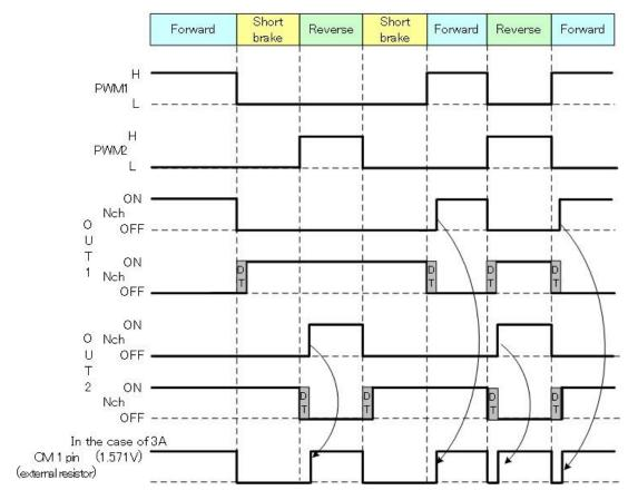
Figure 7.19 High-side current monitoring timing chart
