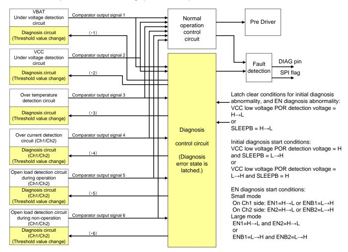
Figure 7.46 Initial diagnosis and EN diagnosis block diagram
