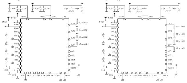
Figure 11.2. OUT pins output delay time measurement circuit diagram
