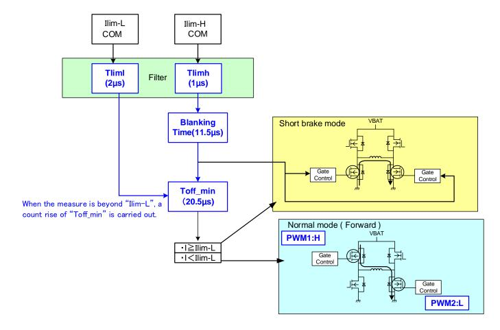
Figure 7.16 Current-limit control circuit operation flowchart
