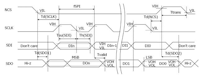
Figure 10.4. SPI communication timing chart
