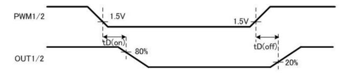
Figure 10.2. Driver output delay time
