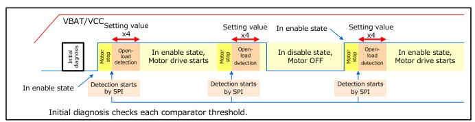
Open-load detection during non-operation: conceptual timing chart
