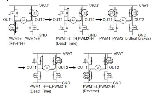
Figure 7.8. Current path for PWM function (reverse rotation, high-side regeneration)
