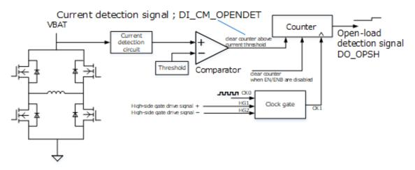
Figure 7.22 Open-load detection during operation: block diagram
