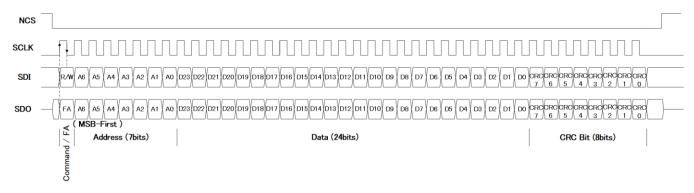
Figure 7.26 SPI communication format
