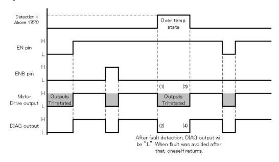
Figure 7.40 Over-temperature detection timing chart
