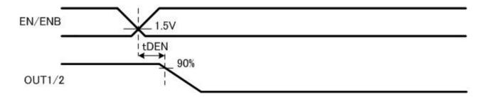
Figure 10.3. Driver output Enable delay time
