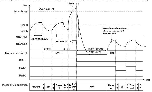
Figure 7.43 Over-current detection operation timing chart 2
