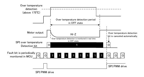
Figure 7.41 Over-temperature detection detailed timing chart
