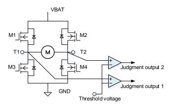
Fig.7.24 Non-operation Load Open Detection Block Diagram
