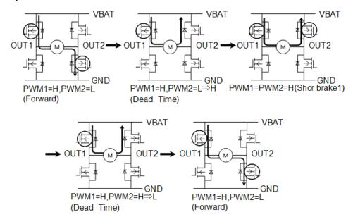
Figure 7.4. Current path for PWM function (forward rotation, high-side regeneration)
