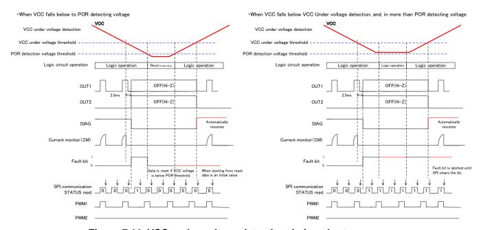
Figure 7.11. VCC under-voltage detection timing chart
