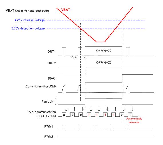
Figure 7.12. VBAT under-voltage detection timing chart
