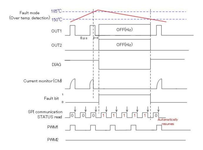
Figure 7.13 Over-temperature detection timing chart
