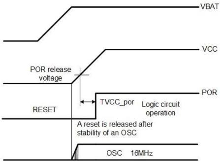
Figure 7.25 OSC circuit starting operation
