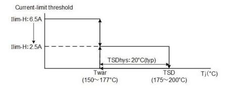
Figure 7.17 Temperature-adjusted current-limit control
