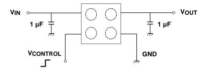
The figure above shows the recommended configuration for using a Low Dropout regulator. Insert a capacitor at VOUT and VIN pins for stable input/output operation. (Ceramic capacitors can be used.)
