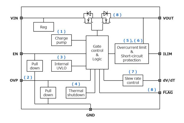
Figure 5.1 Block diagram of the TCKE712BNL
