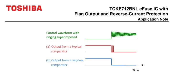
Figure 6.19 Outputs from a typical comparator and a window comparator
