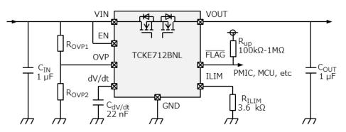
Figure 3.1 Example of an application circuit for the TCKE712BNL
