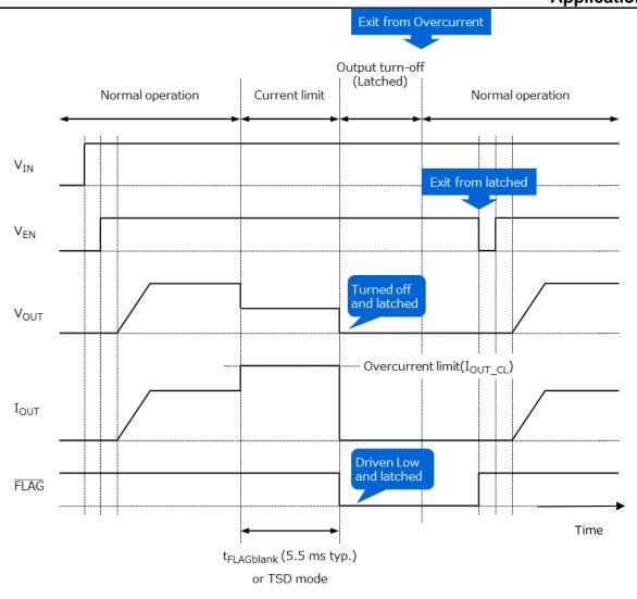
Figure 6.7 Example of an OCP operation
