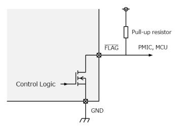
Figure 6.17 Equivalent circuit of the FLAG pin
