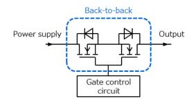
Figure 6.16 Back-to-back reverse-current blocking circuit
