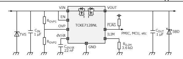
Figure 3.2 Example of an application circuit for the TCKE712BNL with a TVS diode and an SBD
