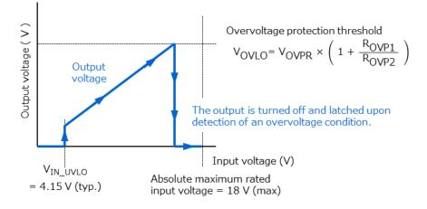
Figure 6.2 Example of an OVP operation
