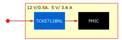
Figure 8.2 Application to SSDs and HDDs
