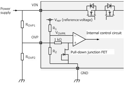
Figure 6.1 OVP circuit
