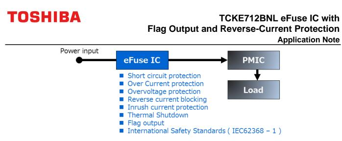
Figure 2.1 Application example of an eFuse IC
