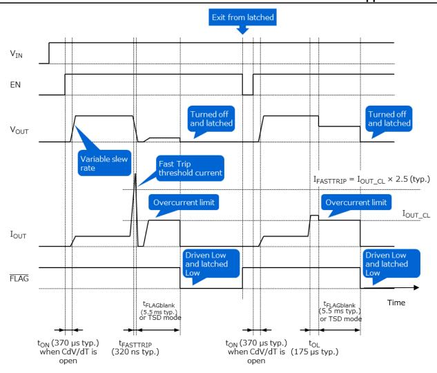
Figure 6.12 Example of short-circuit protection and thermal shutdown operations
