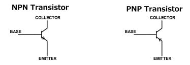
When selecting a transistor product, it is necessary to consider the breakdown voltage (VCEO: collectoremitter withstand voltage), current (IC: collector current), hFE: DC current amplification factor, package / mounting area, etc.
