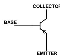
When selecting a transistor product, it is necessary to consider the breakdown voltage (VCEO: collector-emitter withstand voltage), current (IC: collector current), hFE: DC current amplification factor, package / mounting area, etc.
