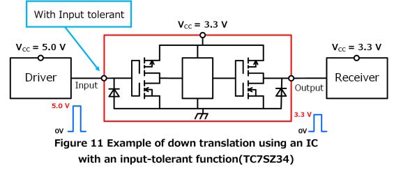
4.6 Case 6: Example of down translation using an IC with an input-tolerant
