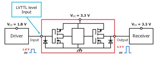
Figure 9 Example of up translation from ultralow voltage using an IC with an LVTTLlevel input (7UL1T34)
