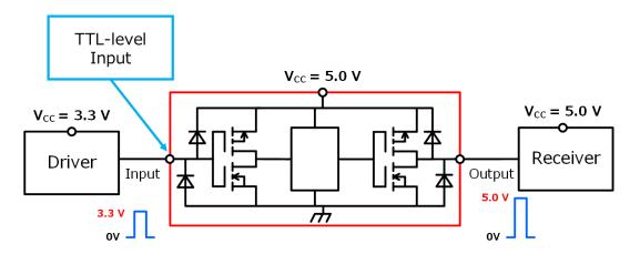
Figure 7 Example of up translation using an IC with a TTL-level input
