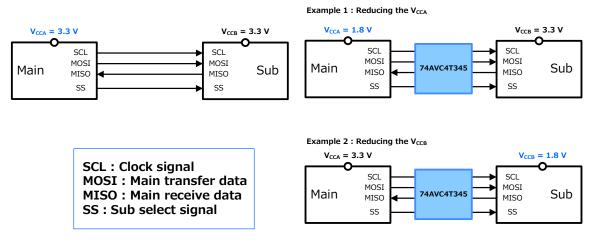
Figure 19 Examples of level-shifting for an SPI interface
