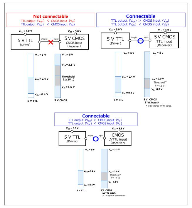
Figure 2 TTL-level inputs (5-V TTL and 3.3-V LVTTL)
