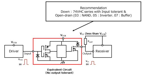
ICs with an output-tolerant function allow both up and down translation to the maximum  $V_{OUT}$  level regardless of  $V_{CCB}$ .
