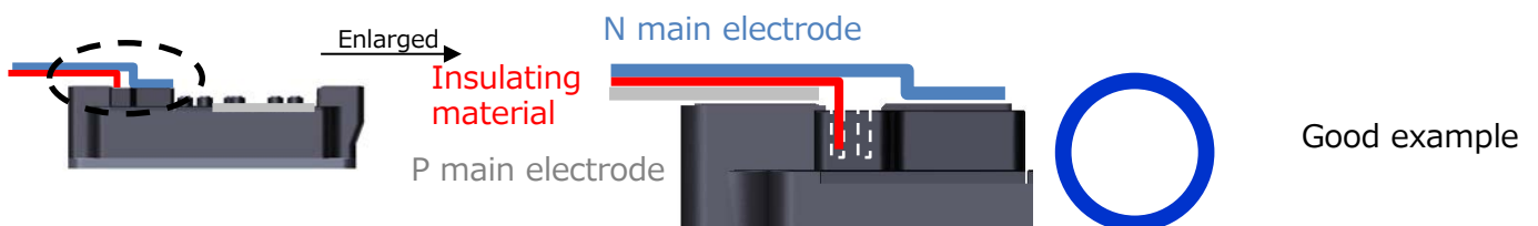
Figure 2.5.4 An example of recommended parallel electrodes and insulation for P and N main electrodes
