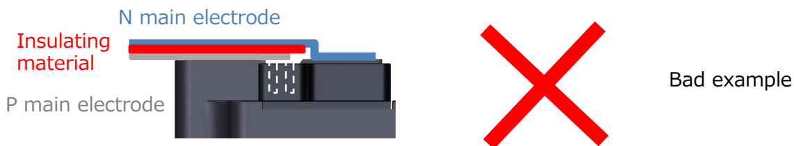
Fig. 2.5.6 An example of insufficient insulation distance between P and N terminals, in the case that the P main electrode moves toward the N main electrode
