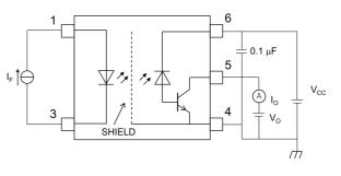
Fig. 12.1.4 I<sub>O</sub> Test Circuit
