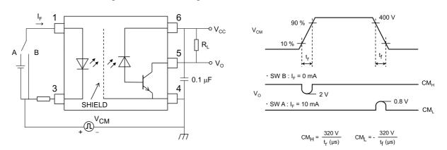
Fig. 12.1.6 Common-Mode Transient Immunity Test Circuit and Waveform
