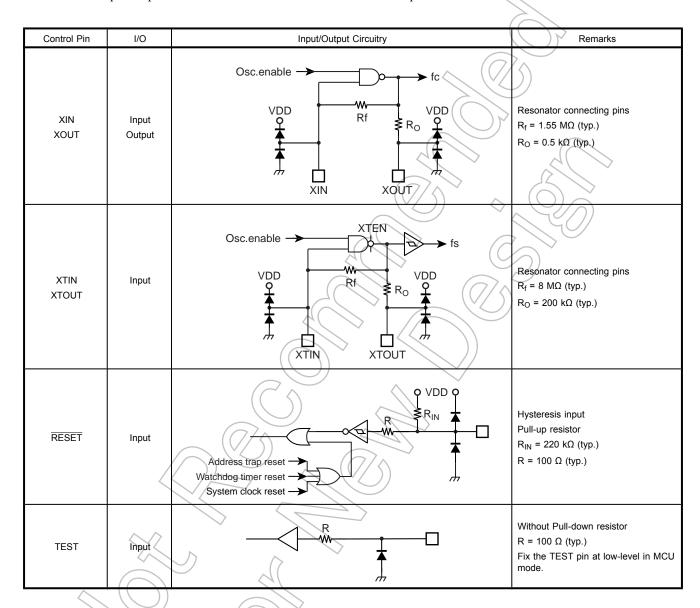
Note: The TEST pin of TMP86FH09/F809/F409NG does not have a pull-down resistor and diode(D1). Fix the TEST pin at Low level in MCU mode.
