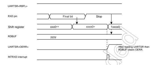
Figure 10-7 Generation of Overrun Error
