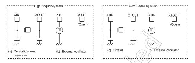
Figure 2-3 Examples of Resonator Connection
