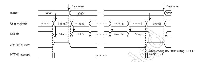
Figure 10-9 Generation of Transmit Data Buffer Empty
