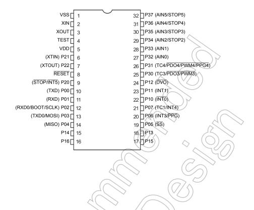
Figure 1-1 Pin Assignment
