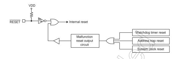
Figure 2-15 Reset Circuit
