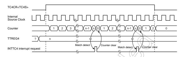
Figure 9-2 8-Bit Timer Mode Timing Chart (TC4)
