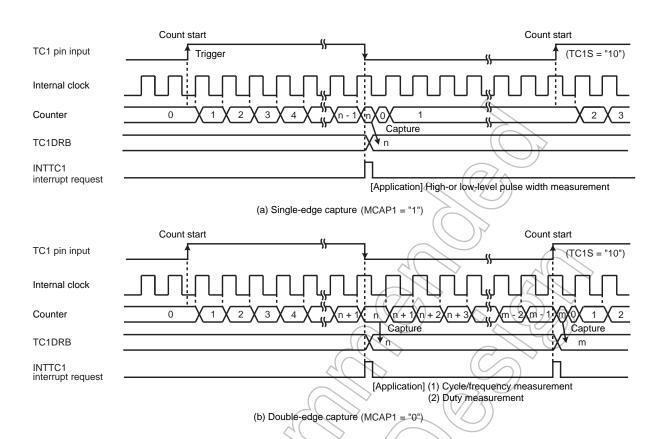
Figure 8-6 Pulse Width Measurement Mode
