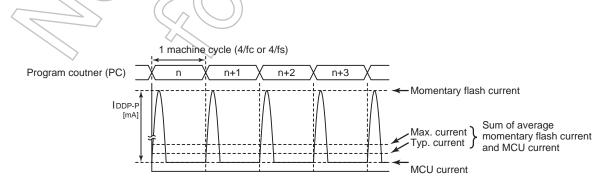
Figure 17-1 Intermittent Operation of Flash Memory
