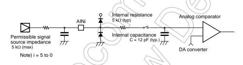
Figure 12-5 Analog Input Equivalent Circuit and Example of Input Pin Processing
