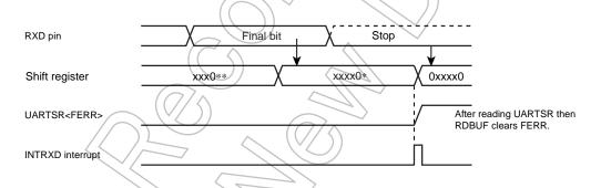
Figure 10-6 Generation of Framing Error
