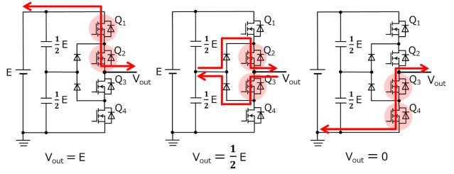
Fig. 3.6 3-Level Inverter Switching Operation
