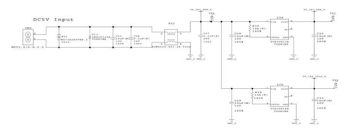
Fig. 4.3 Power supply for CPLD
