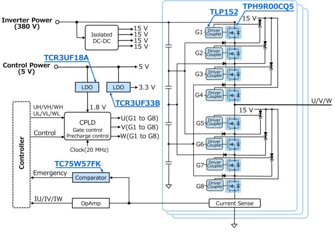
Fig. 4.1 Block Diagram of 3-Phase Multi-Level Inverter using MOSFET
