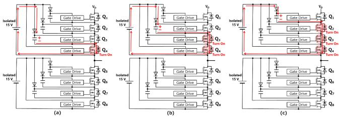
Fig. 4.4 Charging Sequence of Gate Driver Power Supply Capacitors
