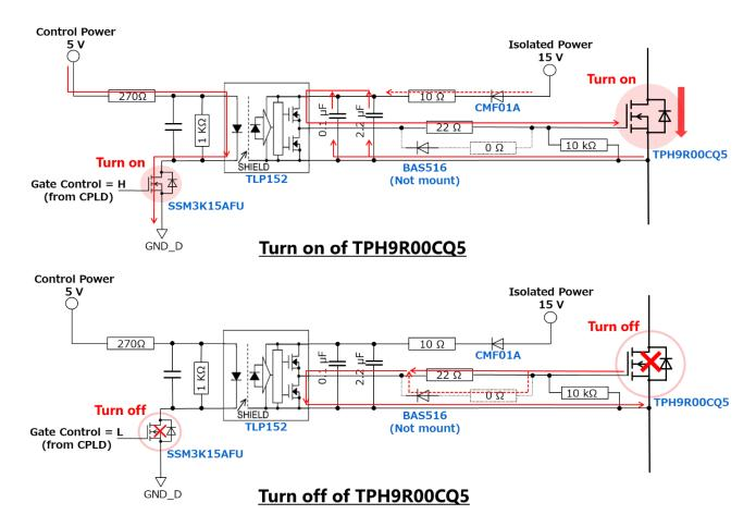
Fig. 4.5 Gate Drive Operation of MOSFET for Inverter Switching
