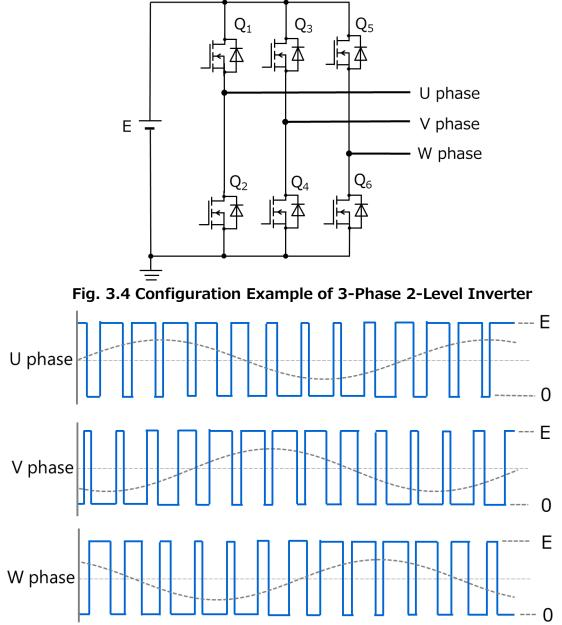
Fig. 3.5 Example of Phase Voltage (Sine Wave) Output of 3-Phase 2-Level Inverter
