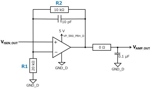
Fig. 4.7 Current Measurement Output Circuit
