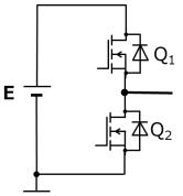
Fig. 3.1 Example of Half-Bridge Circuit
