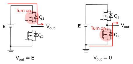
Fig. 3.2 Switching Operation of 2-Level Inverter
