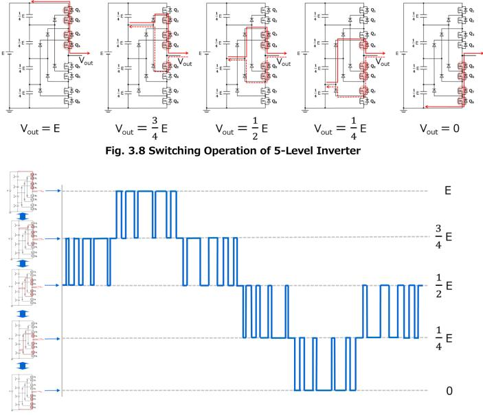
Fig. 3.9 Example of Phase Voltage Output of 5-Level Inverter
